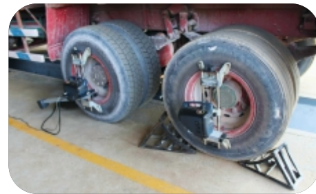
Run out operation for wheel alignment measurement
