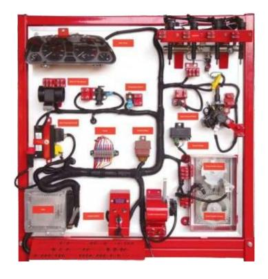
The system comprises all the elements that control the air-fuel ratio, the injectors, the ECU, and all the sensors associated with the control system. Variation of the engine speed allows the measurement of parameters within the system that are speed dependent. This is achieved by changing the rotational speed of the electric motor that drives the unit.
