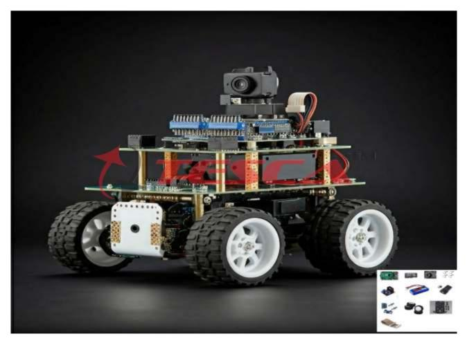
**52072K** AI IOT Robotic Kit; all-in-one solution for building AI , IOT and robotic systems. Tailored for researchers, students, and developers, it includes the powerful Raspberry Pi Model B 4 (4GB) at its core, integrated with a suite of supporting accessories and hardware for robotics and automation applications.
