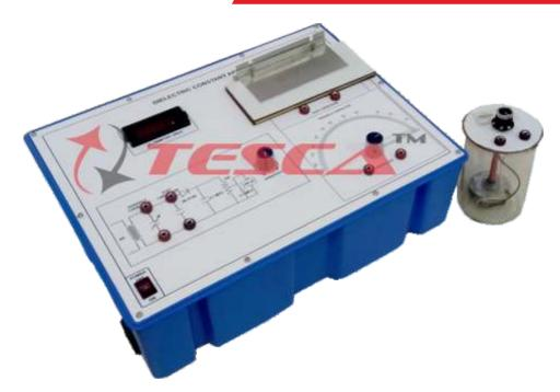
**36396** Experimental Training Board has been designed specifically for to determine the dielectric constant of solid (liquid) different length using slotted section.
