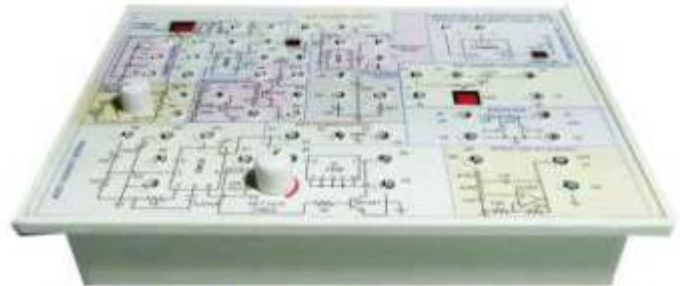
Timer (555) & Frequency (565) application Experiment Panel (P18)
