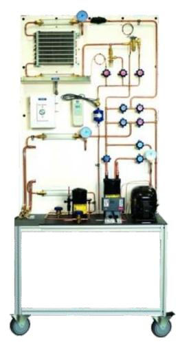
The training unit shows the domestic coolers, Freezers and autonomous air conditioning units with a heat exchanger / condensers Co-axial tube in tube.
