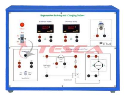
Energy saving and extended mileage are very important for batteryoperated electric vehicles (BEV). Regenerative braking performances are the key for saving energy in BEV's. Trainer introduces Permanent Magnet DC (PMDC) motor based regenerative braking to improve energy efficiency in BEV. The kinetic energy of the motor is returned to the battery system in regenerative charging.
