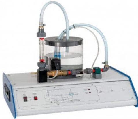
Flow Control: typical controlled system
