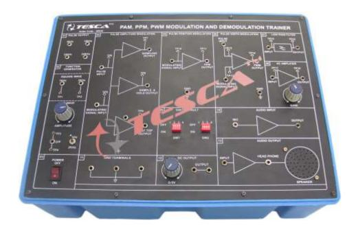
**PAM-PPM-PWM** are the basic Pulse Modulation techniques. The trainer provides complete set up to the students for performing experiments on these techniques. They can study Sampling, Pulse Modulation, Demodulation & Signal reconstruction process. Separate circuits are provided for each technique. The Operating Manual provides technology details and procedure to perform the experiments.
