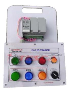
A PLC Input/Output Trainer Kit is an educational and training tool designed to help users learn about Programmable Logic Controllers (PLC's) and their applications in automation. It typically includes the following components:
