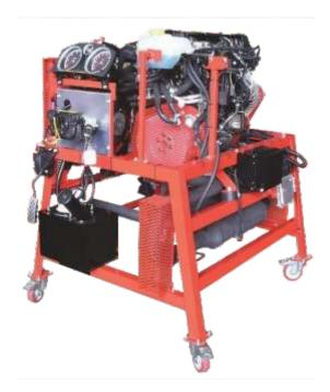
For group or entire class demonstrations, this trainer offers the instructor a complete common rail diesel engine with an engine management system. It is fixed to a moveable, robust steel frame. Together with the ECU and all the sensors and actuators connected to the control system, the system consists of all the components that regulate the timing of the injectors and exhaust emissions.
