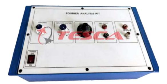
36402 To study of board has been designed specifically for to analyze complex wave (square, sine wave triangular wave etc.) to verify the existence of different harmonics and measure their relative amplitudes.
