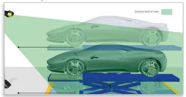
Machine Vision system enhanced HD Camera detects the accurate position of targets on wheels
