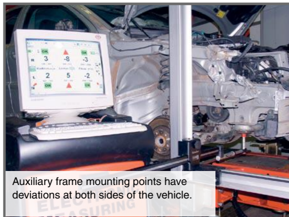
Further checking verifies that the chassis is also within tolerance in other areas except the front.
