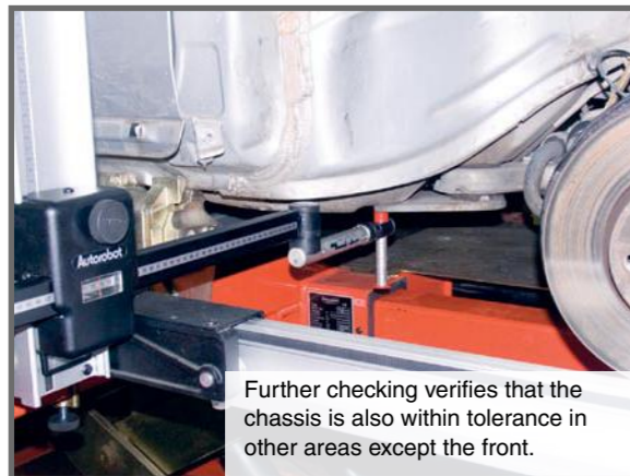
Measuring shows that the McPherson upper end has been pushed back by 4 mm and 2 mm to the side.
