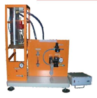
The Tesca Level Control Setup includes an acrylic measurement tank with a Level transmitter, a control valve, an I to P converter, a source tank with a water pump, and all of the necessary flexible pipes for water circulation. The system is installed on a powder-coated metal table top frame. Capacitance or DPT type sensors are used in level transmitters. DELTA PLC with USB interfaces make up the electronic panel.
