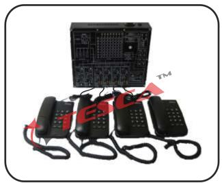
EPABX Trainer is a Microprocessor based system designed to help the students to understand the basic concept and working of a Telephone Exchange. All the components are mounted on a single PCB in functional blocks and have various Test points to monitor all kinds of telephonic signals.
