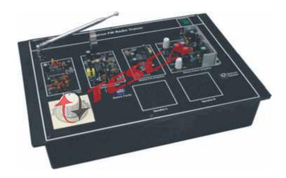
**Stereo FM Radio Trainer** is designed to cover the fundamental aspects of the subject. This is Student friendly and self contained, having all the basic required circuits and control on board. FM detection is described in the manual and covered in the experiments. Student trouble shooting work is included through switched faults in this trainer. This forms a complete training package of Stereo FM Radio trainer.
