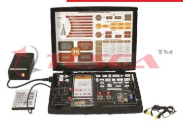
**10903D** Understanding 4G VoLTE Smart Phone is a unique, self contained, easy to operate, training and platform that demonstrates the complete study and working of a 4G Dual SIM VoLTE handset to understand the fundamentals of Smart phone.
