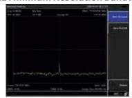
Digital IF technology offers a minimum bandwidth of 10Hz, allowing excellent signal resolution when separation of closely spaced signals is required.
