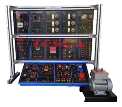
46627 Industrial Installation Trainer is a rouged training system for the Electrical laboratories mounted on Aluminum profile rack with sturdy table top flat panel. Each panel has ABS molded plastic sturdy enclosure with 4mm shrouded connectors showing circuit diagram & its connection tag numbers for easy understanding and connections. The product helps you to get fully acquainted with the basic concepts and functioning of an Industrial Installation Trainer.
