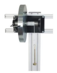
**Description:** This self-contained unit is designed to demonstrate the Second Law of Motion and principles of energy storage. It includes a steel flywheel and various accessories to facilitate hands-on learning and experimentation.
