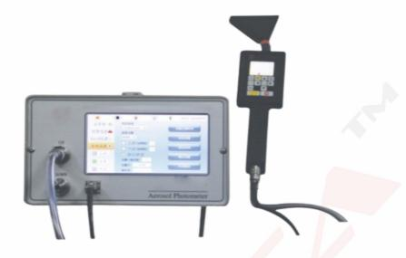
Aerosol Photometer is the advanced digital, linear aerosol photometer using the light scattering method. The basic function of this Aerosol Photometer is to sample air or other gases and report the mass concentration of particulates in the sample. The most common application is to detect the leaks and reflect the integrity of high efficiency filter systems.
