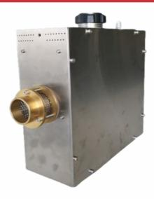
Aerosol generator (thermal) adopts the principle of evaporation and condensation, with a particle size distribution range of 0.1~0.3um, high concentration, continuous stability, suitable for various small air purification units and large clean room air conditioning purification systems (flow range 14 ~2000m3/Min).
