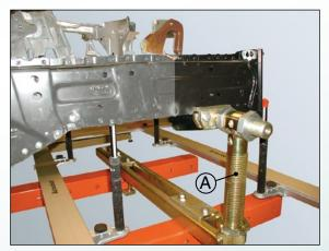
The support/jig system (A) will hold a new part in its correct position as the vehicle is pulled to it. Shown here, the new frame end is held in place during straightening and after, for welding.
