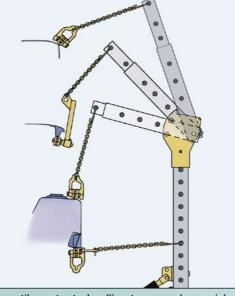
Versatile, patented pulling tower makes quick work of straightening. Adjusting the correct pulling angle takes seconds. Straight upward pulls are easy thanks to the telescopic upper beam which can be set in three positions (A, B, C).
