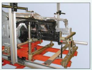
All new parts can be correctly positioned on the front of the car with the multi-purpose support/jig system. 3D measuring system ensures top-quality results.
