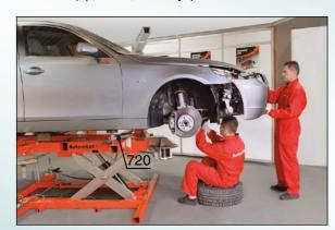
Use the XLS+ as a lift for reassembling parts or for other repairs. It allows easy access to the front end, engine and wheel assemblies.
