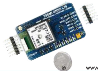
T1123 7Semi L89HA Breakout Multi-GNSS Engines for GPS, IRNSS, GLONASS, BeiDou, Galileo and QZSS
