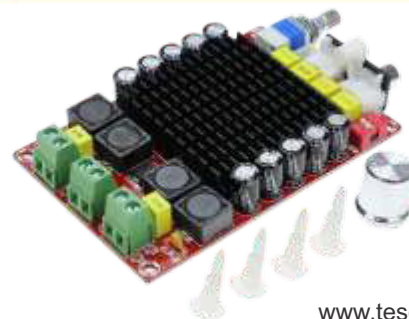
T1062 XH-M510 TDA7498 DC14-32V High Power Digital Power Amplifier Board
