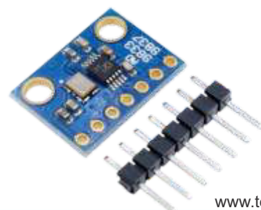
T1052 GY-9833 AD9833 Programmable Sine Square Wave DDS Signal Generator
