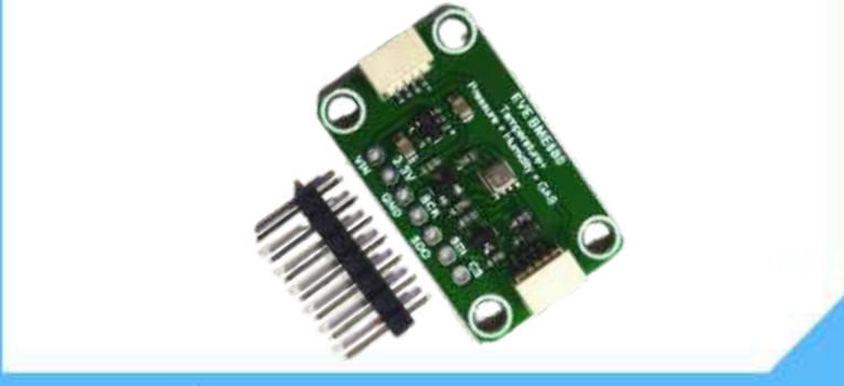
T1132 7Semi SCD40 CO2, Temperature and Humidity Sensor Breakout I2C
