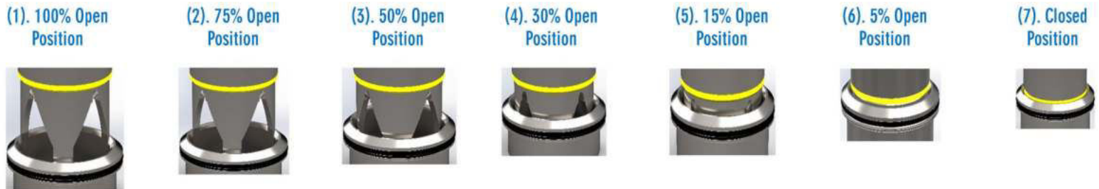
Figure 1: V-Port Open Positions At Incremental Percentages
